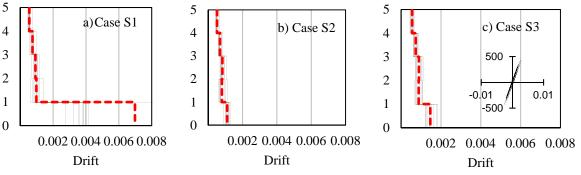
Figure 10. Drift profiles for Sa/g = 0.30; hysteresis cycle in kN and m.
