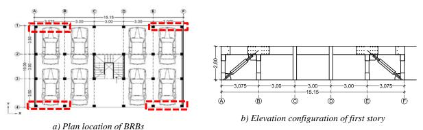
Figure 4. Location of buckling-restrained braces. Case S3.
