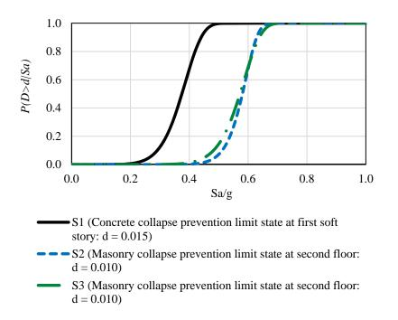
Figure 13. Fragility curves for collapse prevention limit state. Cases S1, S2 and S3.
