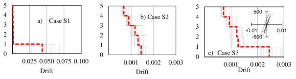
Figure 11. Drift profiles for Sa/g = 0.41; hysteresis cycle in kN and m.
